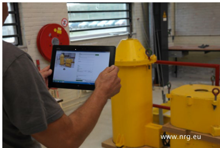
FIG. 49. Digital track and trace system of all disposed components and materials, using a tablet device for entering data and photographs into the database. (Reproduced courtesy of NRG.)
