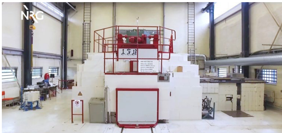
FIG. 47. The Low Flux Reactor of NRG with shielding of stacked concrete blocks (the facility for BNCT medical research is on the right). (Reproduced courtesy of NRG.)
