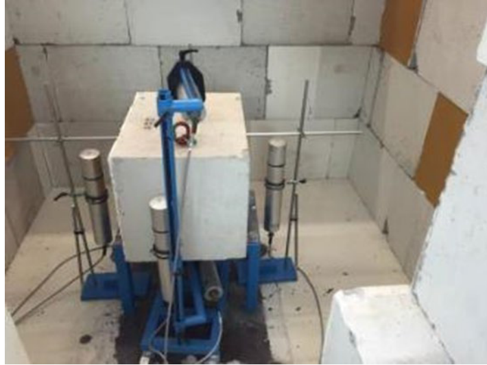
FIG. 52. Shielded measurement setup. (Reproduced courtesy of NRG.)
