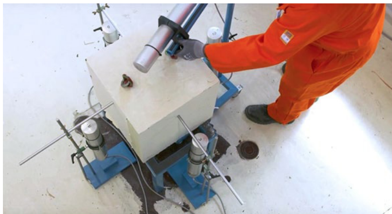
FIG. 51. Measuring device for determination of activation in barite concrete shielding blocks. (Reproduced courtesy of NRG.)
