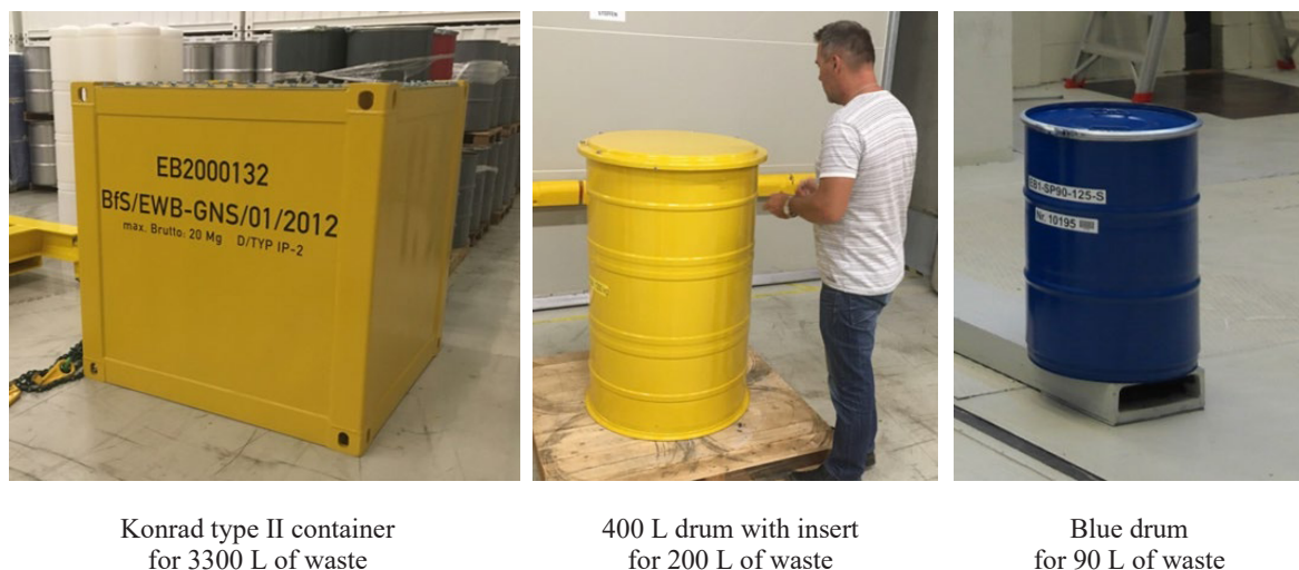
FIG. 50. Three types of waste packages used during decommissioning. (Reproduced courtesy of NRG.)
